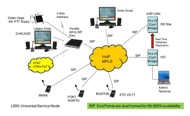
Figure 2: IP based Hoot-n-Holler Network
