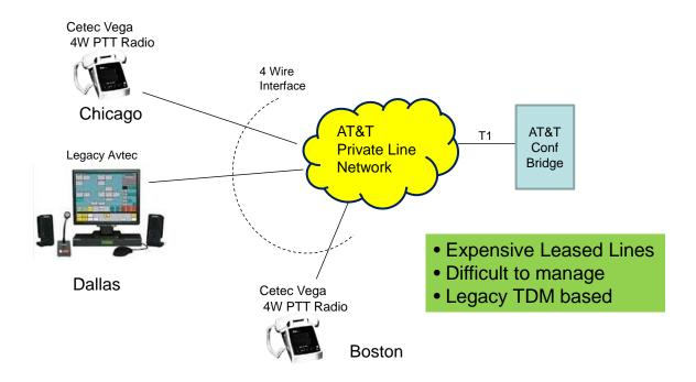
Figure 1: Traditional Analog/TDM based Hoot-n-Holler Network
